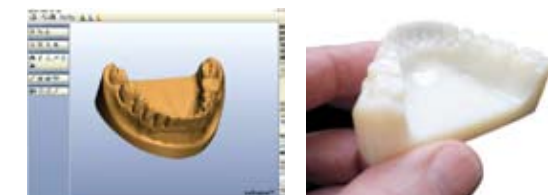
From a digital file to a 3 dimensional dental model
